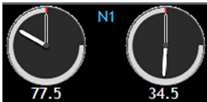
Fig 4: Example of hollow pointers used to show N1 command, with filled pointers to show actual N1.
